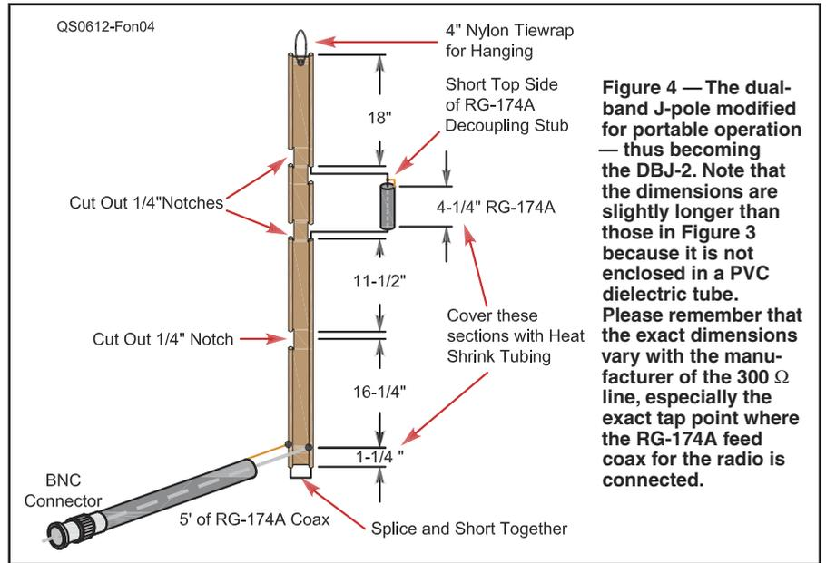
**Figure 4 — The dual-band J-pole modified for portable operation — thus becoming the DBJ-2. Note that the dimensions are slightly longer than those in Figure 3 because it is not enclosed in a PVC dielectric tube. Please remember that the exact dimensions vary with the manufacturer of the 300  $\Omega$  line, especially the exact tap point where the RG-174A feed coax for the radio is connected.**
