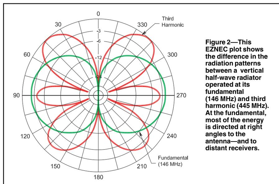
Figure 2—This EZNEC plot shows the difference in the radiation patterns between a vertical half-wave radiator operated at its fundamental (146 MHz) and third harmonic (445 MHz). At the fundamental, most of the energy is directed at right angles to the antenna—and to distant receivers.
