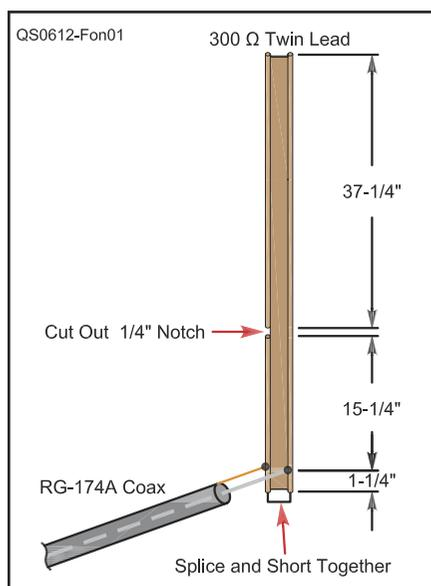
Figure 1 — The original 2 meter ribbon J-pole antenna.
