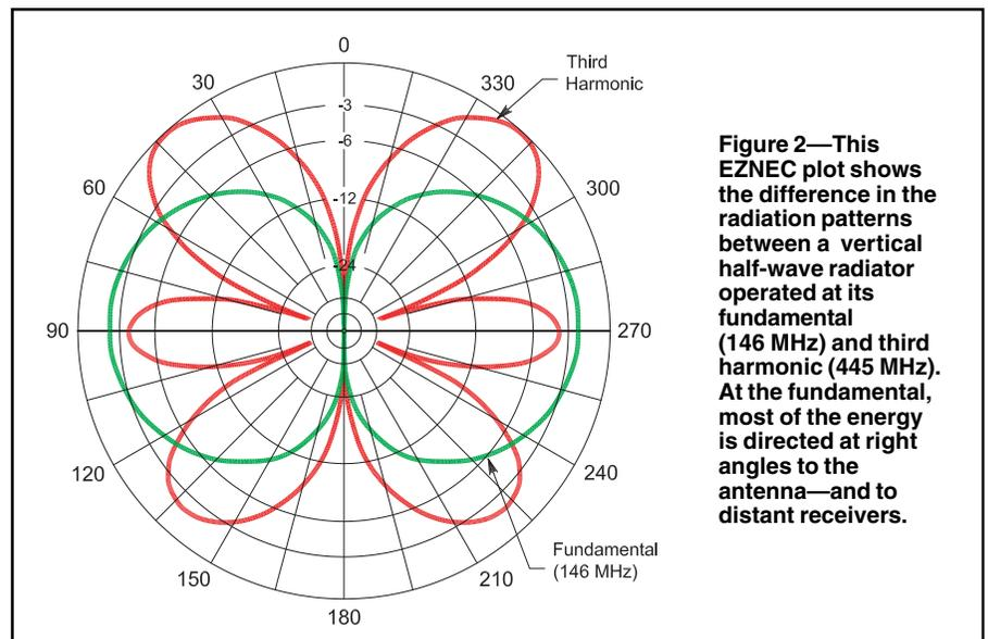
Figure 2—This EZNEC plot shows the difference in the radiation patterns between a vertical half-wave radiator operated at its fundamental (146 MHz) and third harmonic (445 MHz). At the fundamental, most of the energy is directed at right angles to the antenna—and to distant receivers.
