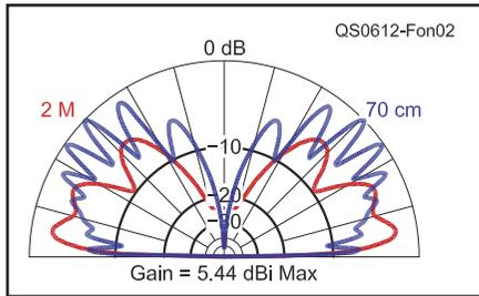
**Figure 2 — Elevation plane pattern comparing 2 meter J-pole on fundamental and on third harmonic frequency (70 cm), with the antenna mounted 8 feet above ground. Most of the energy at the third harmonic is launched at 44°.**
